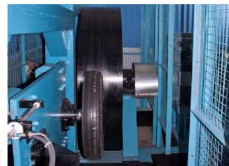
tels 10K50 is designed and developed to test the performance of tyres under test at rated load and rated speed for a set duration of time. In endurance test tyres is run at set constant speed and load is increased on it stage-wise. In case of Load/Speed performance test a constant load is kept and speed is increased stage wise.
